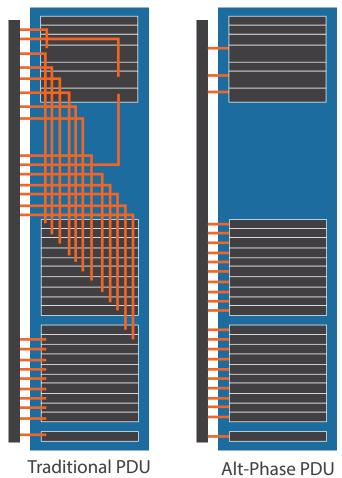
Server Technology has patent pending unique method of distributing the alternating phase power to each outlet. Instead of using wires, our products use a multi-layer circuit board to separate the phases. Each outlet contacts a different trace within the board to distribute the proper phased voltage. This helps to reduce heat build-up in the PDU, lessens the human error during manufacturing and finally creates a cleaner design to reduce the physical size of the product.
