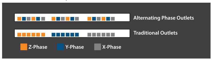
Alternating phase PDUs are also a great choice for Basic PDUs where there is no current measurement or display on the unit to assist with load balancing. Installers can plug in servers from the bottom to top of the rack with less risk of blowing a breaker since there are no dedicated branches across the length of the PDU.
